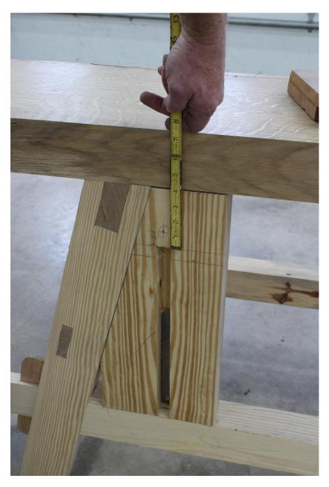
The chop needs to be at least 2  $\frac{1}{2}$ " thick (the one pictured is 2  $\frac{1}{2}$ "). The rest of the chop dimensions are the same as given in the bench plans. Leave the vise square, cut it to shape after the mortise and screw have been installed.
