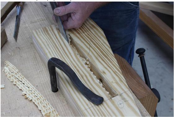
Clean the bottom of the mortise up with a router plane. The lower part of the mortise has an iron bearing plate that installs with a single screw.
