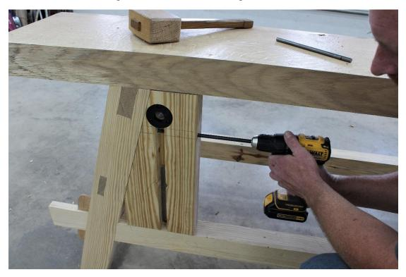
The vise chop can now be cut to whatever shape you desire and reinstalled. The acetal bushing can also be installed.
