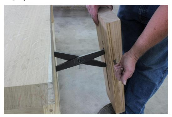
With the chop on and flat against the bench, insert the bit used to bore the vise screw hole into the screw hole and tap with a mallet. This will give you a perfectly aligned layout on the vise support.
