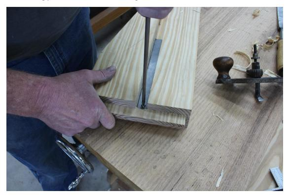
The pivot pin holes are 3/8" in diameter and located ¾" from the top edge of the mortise and 13/16" in from the face. BC recommends boring these on a drill press but the angled side of the vise support prevents it in this case. I use a long 3/8" bit and a scrap of wood clamped and aligned to the pivot layout line. This gives you a reference edge to guide you drill bit. Bore halfway from either side meeting in the mortise.
