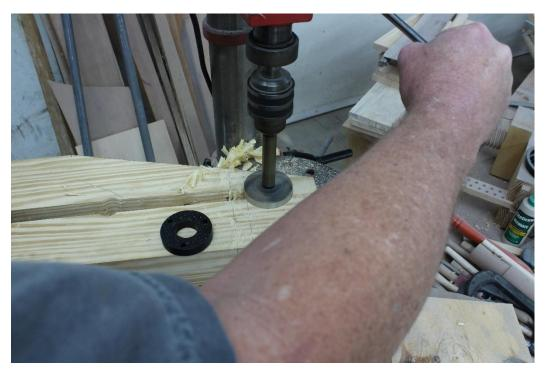
There are several ways to help center the vise screw in the holes in the chop and support. I wrapped several layers of masking tape on the screw in a couple of places and it worked well.
