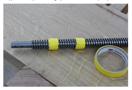
With the tape in place insert the screw into the vise and snug the nut on the back by hand.
