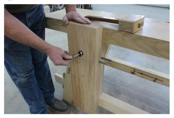
Remove the vise chop from the vise support and remove the support from the bench. There is an acetal bushing that is installed on the face of the vise support to help guide the screw. This hole is bored first to about  $\frac{1}{2}$ " deep and the 1  $\frac{1}{2}$ " vise screw hole is bored the remainder of the way thru the vise support.
