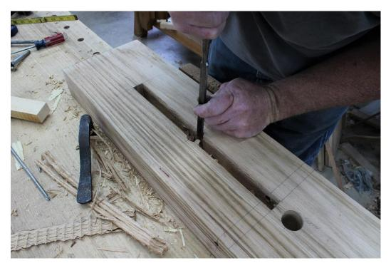
I cut the reliefs in the sides of the mortises for the center pivot pin with a gouge, BC recommends boring a 1 %" hole at the center of the mortise. I forgot this step!
