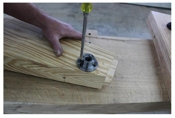
Reinstall the vise support and using the long 3/8" bit bore thru the pivot pin hole into the leg an inch of so. This will allow the pin to extend into the leg and help distribute some of the pressure
