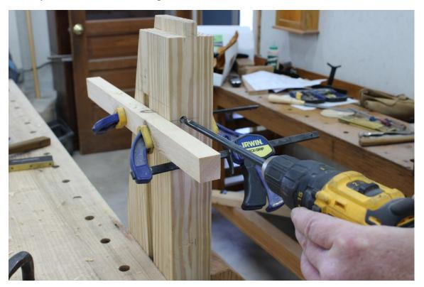
Reinstall the vise support in the bench and measure the distance from the top of the crisscross mortise to the top of the bench. Add about  $\frac{1}{2}$ " to this measurement and that will be where the top of the vise chop mortise will need to be located from the top edge of the chop. The added  $\frac{1}{2}$ " will give you a little extra chop length above the benchtop. This can be marked and cut to final length after the vise is mounted.
